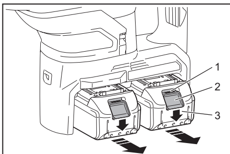
► 1. Red indicator 2. Button 3. Battery cartridge
